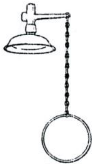
A safety shower with pull chain
